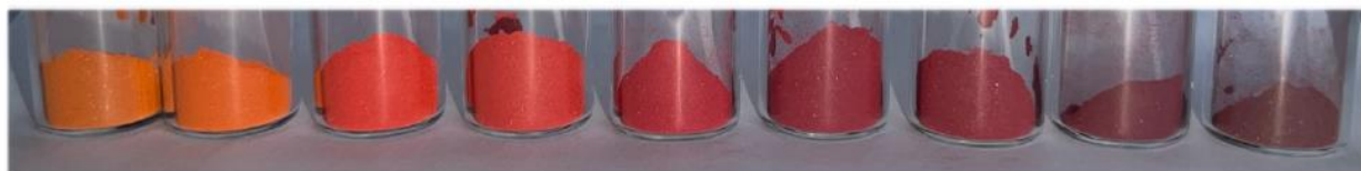
Figure 1. Variation of the hue of the pigments \text{CdS}_{1-x}\text{Se}_x pigments increasing the selenium amount (from the left).
