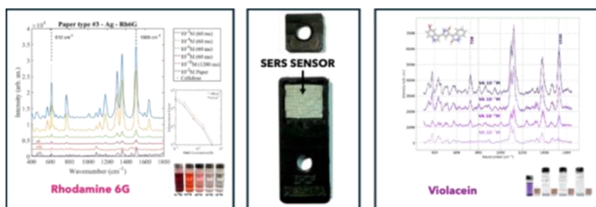
Figure 1. Detection of Rhodamine 6G at different concentrations (left panel), prototype of the SERS sensing system (center panel), and detection of violacein at different concentration levels (right panel).
